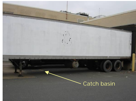
Truck loading/unloading operations at this dock occur over a stormwater catch basin, increasing the potential for oil and spills to enter the system.
